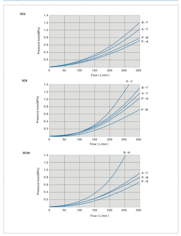
**06 Specification** Performance curve ( Measured at  $\upsilon$  =41mm²/s and t=50°C )
